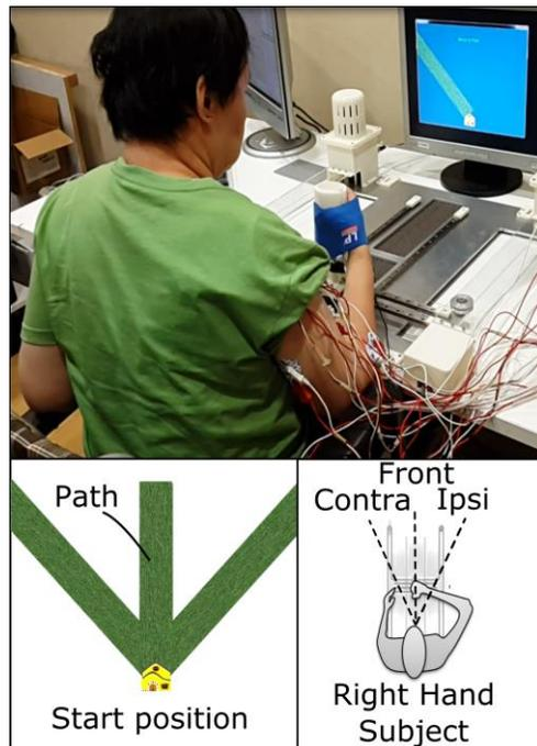
**Figure 1(Top)** Subject using H-Man robot for assessment task. **(Bottom)** Visual stimuli used for the assessment with the directions explained.
